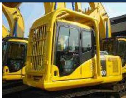
Engins à cabine renforcée (type FOPS –falling objects protective structure).
