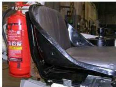
**Fig. 12. Dry-powder extinguisher installed on the operator's workplace**
