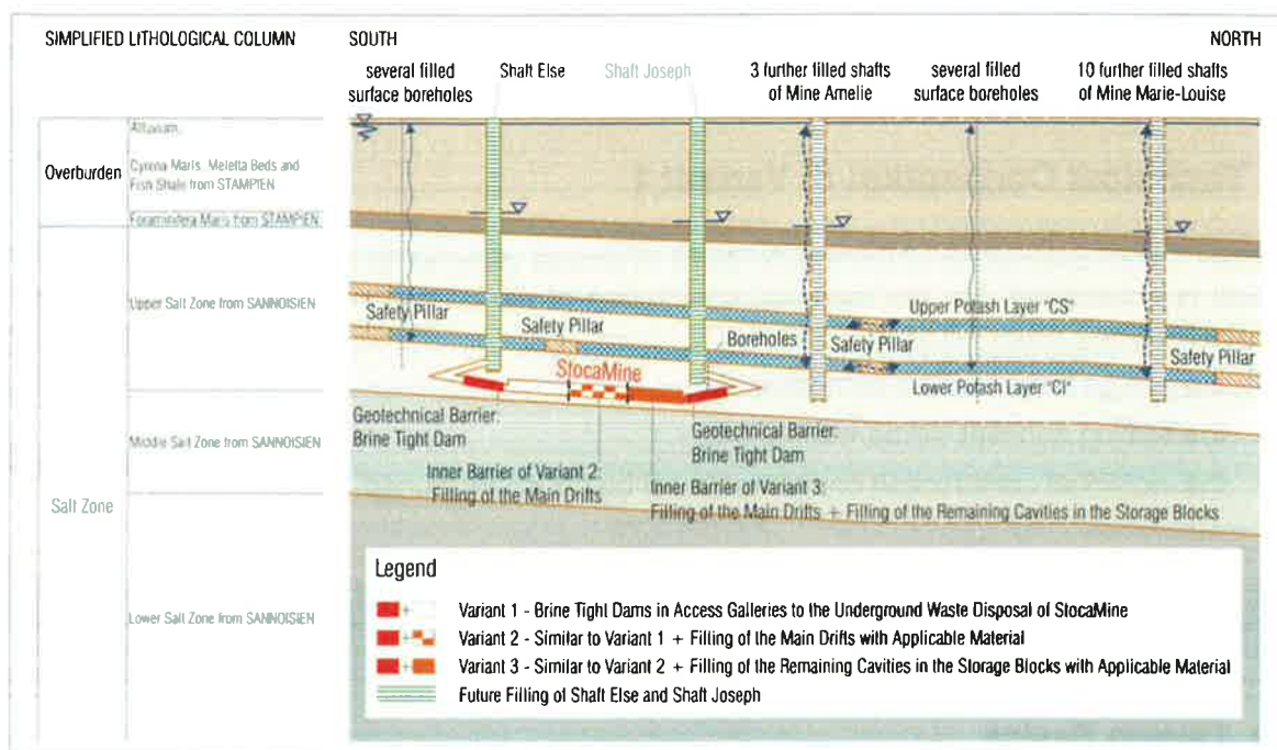
Figure 2 Schematic Overview of the Safety Concept "Multi Barrier System" for the Underground Waste Disposal of StocaMine
